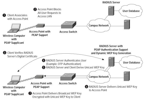
8 Client and Access Point Activate WEP and Use Unicast and Broadcast WEP Keys for Transmission
