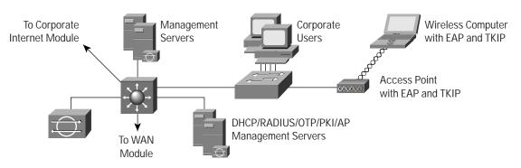
EAP access in the medium WLAN design has wireless access points connected to the existing Layer 2 access switch in the medium-campus module. RADIUS and DHCP servers are also located in the campus module, but off a distinct Layer 3 subnet on the central-campus Layer 3 switch. The wireless EAP users will require DHCP and RADIUS authentication services to access the medium-campus network. If the medium network is a branch office, the DHCP and RADIUS servers may reside at the corporate office.
