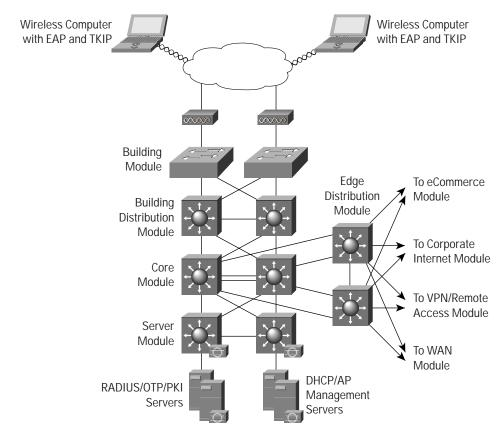
EAP access via the wireless network takes advantage of three components from the SAFE enterprise architecture:
