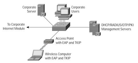
Cisco EAP access in the small WLAN design has wireless access points connected to the existing Layer 2 access switch in the small-campus module. The wireless EAP users require DHCP and RADIUS authentication services to access the small-campus network. Because of the single-site nature of small networks, the RADIUS and DHCP servers reside locally connected to the Layer 2 switch in the campus module.
