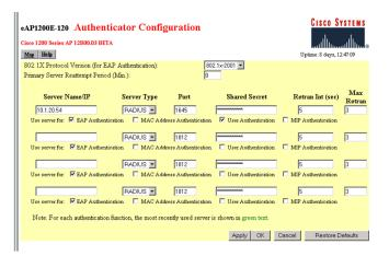
Figure A-2 illustrates the security configuration for an EAP access point. "Full Encryption" (wired equivalent privacy [WEP]) is mandated by the access point; in addition, the access point allows network EAP as the only authentication method. EAP types configured for this deployment included Cisco-EAP (LEAP), Protected EAP (PEAP), and EAP-Transport Layer Security (EAP-TLS).
