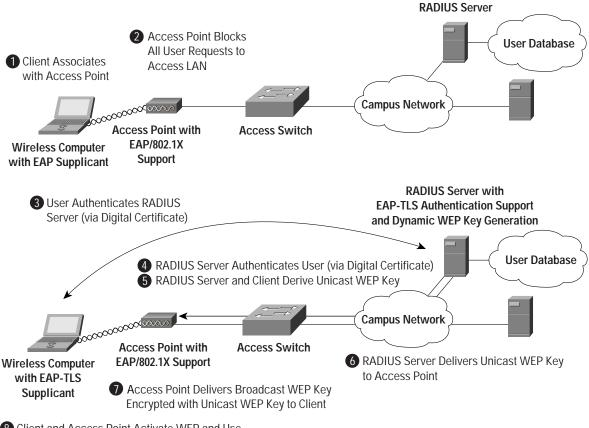
8 Client and Access Point Activate WEP and Use Unicast and Broadcast WEP Keys for Transmission
