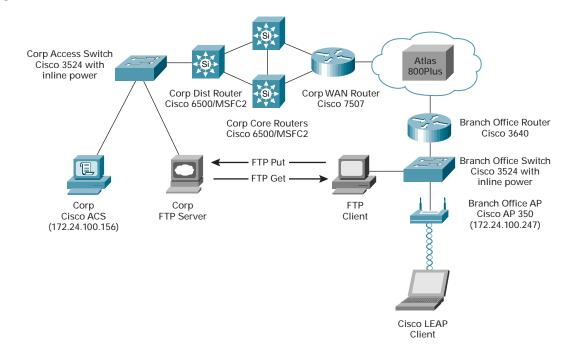
The WAN is simulated using an Adtran Atlas 800Plus WAN circuit emulator. A T1 is provisioned for use between the main WAN router and the branch office router. To simplify the testing, only one 64-kbps channel is enabled on the routers.
