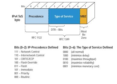
Figure 6 IP Precedence in an IPv4 Header
