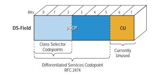
Standard 802.1x RADIUS packets are considered network control packets, so to maintain consistency with other Cisco products and standards, 802.1x RADIUS frames are marked as DSCP value AF31. For some perspective, the AF31 marking places 802.1x RADIUS frames in the same class as voice over IP (VoIP) call control packets.
