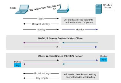
Figure 2 Authentication Process with 802.1x
