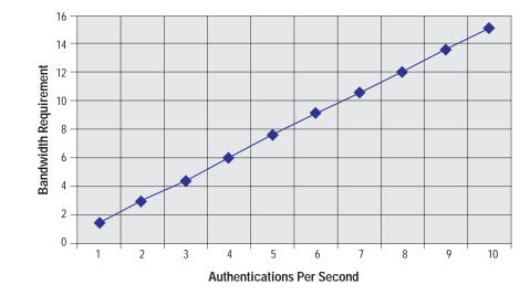
Figure 8 Authentication Rate vs. Bandwidth Requirement
